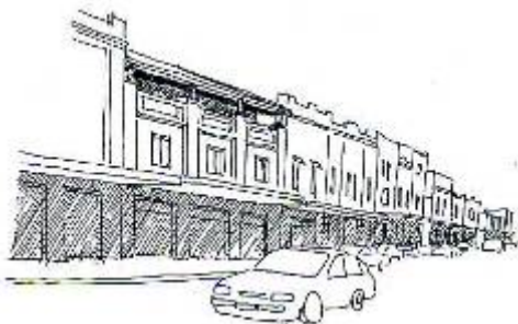
Parapet becomes balustrade for upper storey
