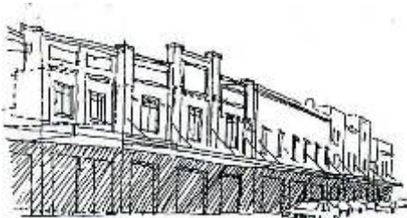
Parapet of single storey building raised to allow for second storey addition
